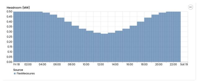
The graph shows that the capacity of the grid is at full disposal for the battery when there's no sun (thus no PV generation), while at noon the battery can only discharge at 280kW max.
