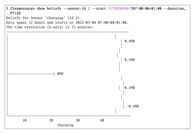
Here, negative values denote output from the grid, so that's when the battery gets charged.
