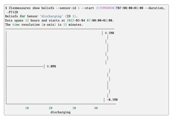
Here, negative values denote output from the grid, so that's when the battery gets charged.
