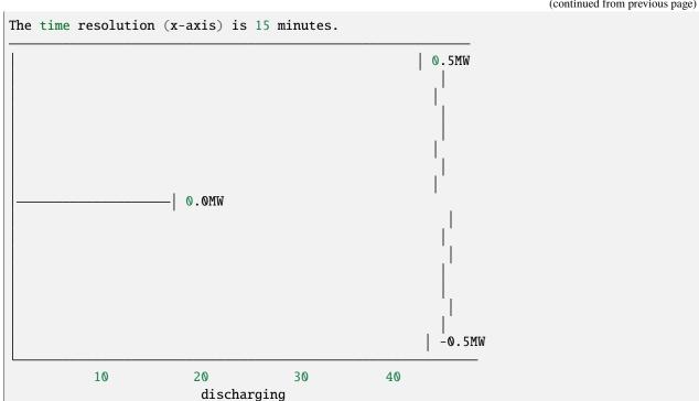
Here, negative values denote output from the grid, so that's when the battery gets charged.
