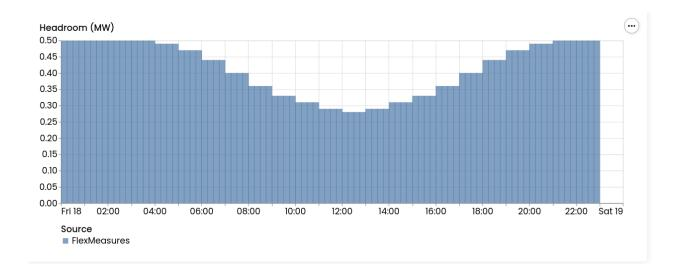
The graph shows that the capacity of the grid is at full disposal for the battery when there's no sun (thus no PV generation), while at noon the battery can only discharge at 280kW max.
