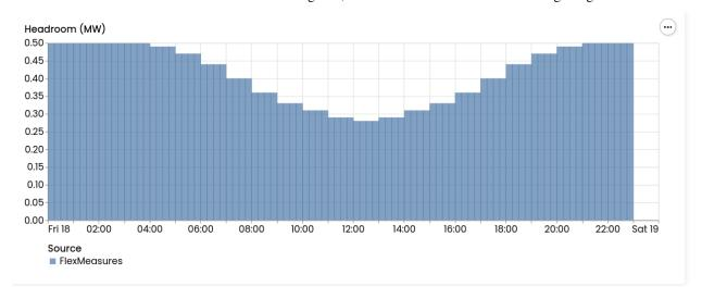
The graph shows that the capacity of the grid is at full disposal for the battery when there's no sun (thus no PV gener-
