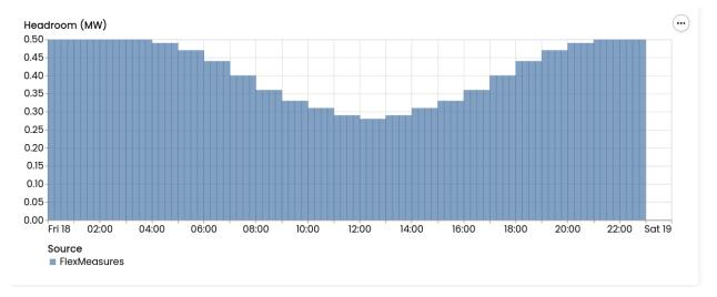
The graph shows that the capacity of the grid is at full disposal for the battery when there's no sun (thus no PV gener-
